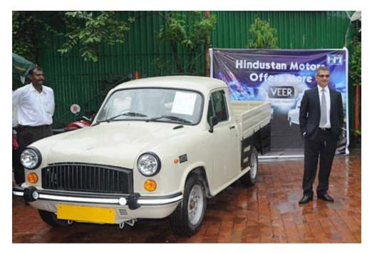
The Veer is built on the tried and tested Ambassador platform, incorporating changes in transmission and suspension systems required for a load carrier. The vehicle is available in both diesel (BS III) and CNG (BS IV) versions and in two models – Veer and Veer LX. While Veer has a separate load tray, Veer LX's load tray is seamlessly integrated with the front cabin.
