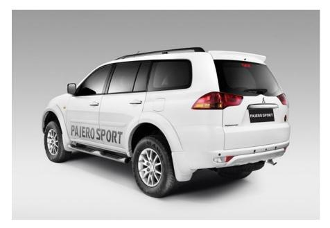
Mitsubishi Pajero sport is powered by 2.5 L Common rail turbo charged diesel engine which makes 176 BHP of power and 400 Nm of torque. This engine is mated to a 5 speed manual transmission. Mitsubishi assemble the Pajero sport at the Hindustan Motors Tiruvallur plant near Chennai. Mitsubishi Pajero sport is priced at RS 22.56 Lakhs (Ex-showroom Delhi). The price tag of Pajero Sport is little expensive compared to the rivals like Toyota Fortuner and Hyundai Santa Fe.
