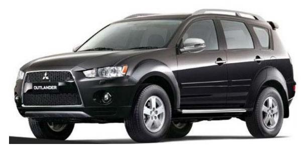
There isn't an engine change in the limited edition. It is powered by 2.4 litre petrol engine with 168bhp of power and 226 Nm of torque coupled to a 6-speed CVT transmission. It offers ABS with EBD and active stablity control. It also comes with four-wheel drive capability, available at the flick of a dial.
