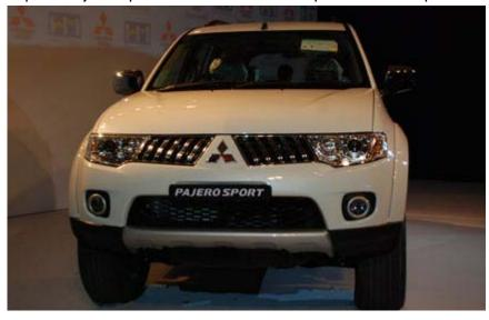
provides better fuel efficiency. It is marked by strong specifications like maximum power of 178 PS. maximum torque of 400 N-m, ondemand super select 4 facility, WD rear stabilizer and a turning radius of 5.6 meters.
