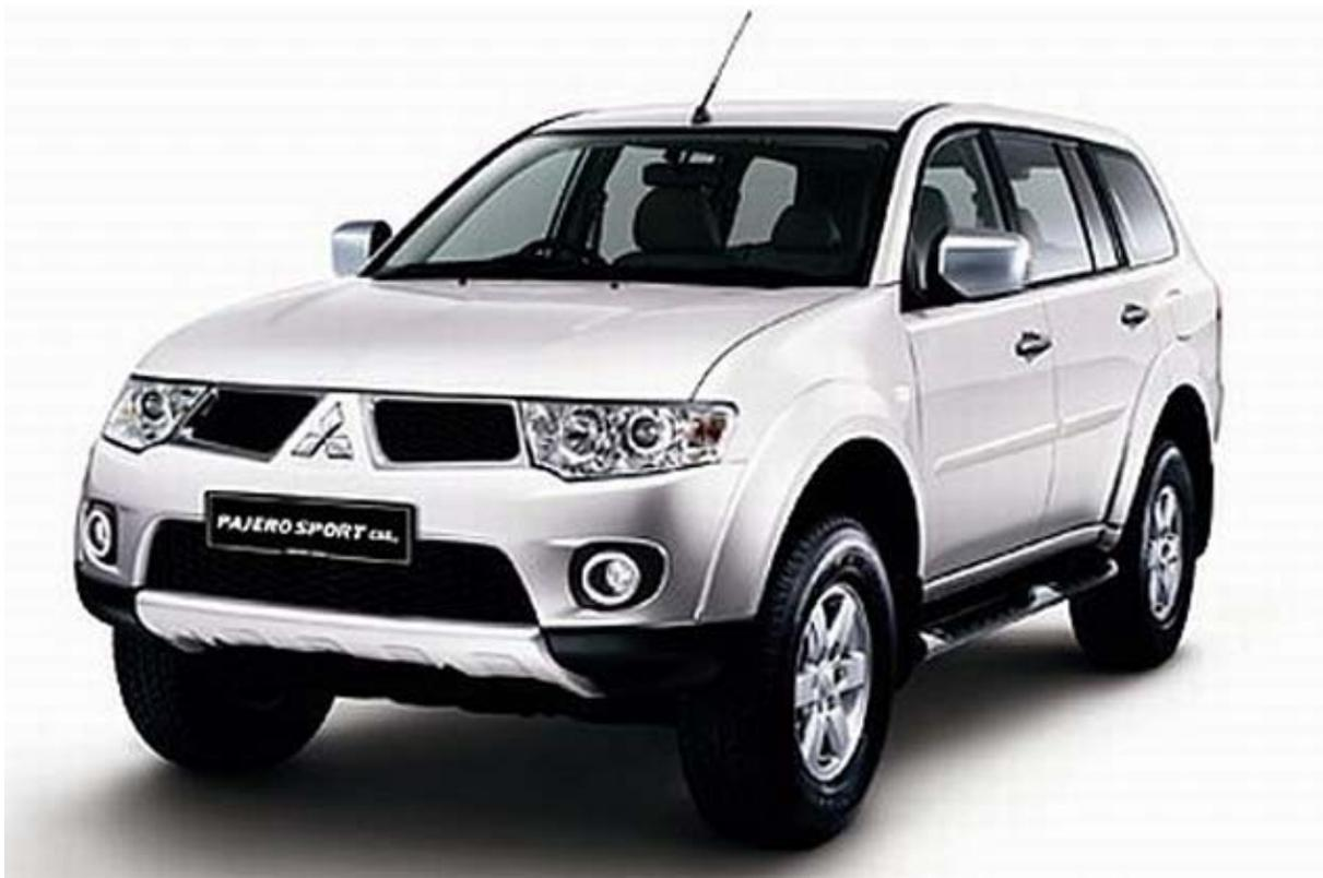
Pajero Sport offers best in class power and torque with VG turbo engine and yet provides better fuel efficiency. It is marked by strong specifications like maximum power of 178 PS, maximum torque of 400 N-m, on-demand super select 4 WD facility, rear stabilizer and a turning radius of 5.6 meters.
