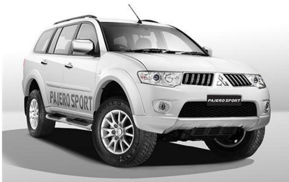
It is powered by a 2.5-litre diesel engine which can produce 176 BHP of power at 4000 RPM and 400 Nm of torque at 2000 RPM and the engine is mated to a 5-speed manual gearbox.
